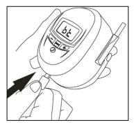
There are three different ways music can be piped in the earmuffs, i.e. FM radio (frequency band of  $88 \sim 108$  MHz), MP3 via the 3.5mm audio jack, and Bluetooth connected to a smartphone.
